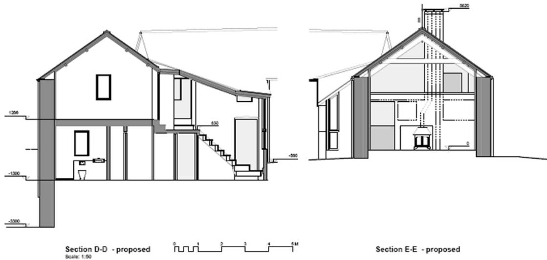
A new chimney at the junction of the original barn with the later addition allows for biomass heating and thermal store. This is positioned to minimise shadowing of solar collector arrays either side. The existing windows are mainly metal-framed additions. Being an
